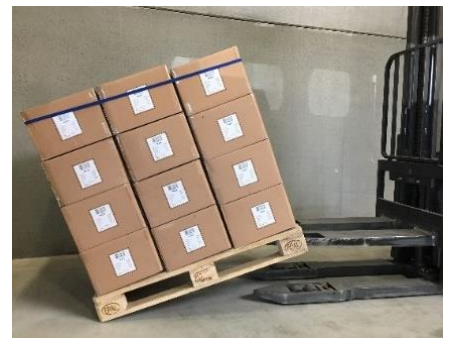
Allows a 30° angle of inclination of the pallets with a single suitable elastic
