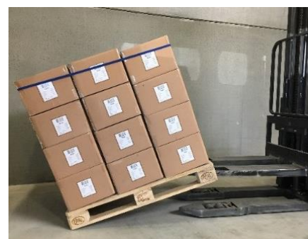
Allows a 30° angle of inclination of the pallets with a single suitable elastic
